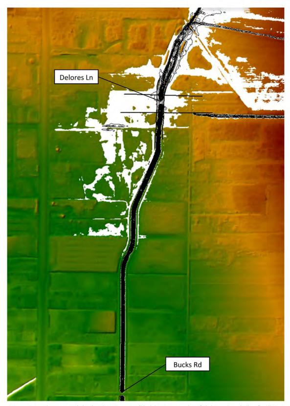
Figure 6. Inundation Areas (white) and DxV Contours (black lines, set to value of 1) show minor shallow flooding outside of channel banks with no DxV outside of channel banks between Delores Ln and Bucks Rd.
