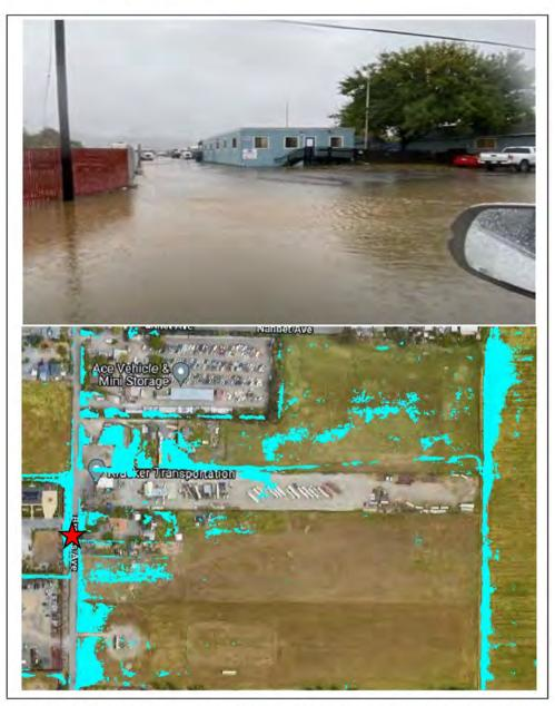
Figure 14. Comparison of Observed Flooding and Model Results. The Star Shows Where the Picture was Taken (looking east) (Image taken on Oct 24, 2021, 3:41 PM)
